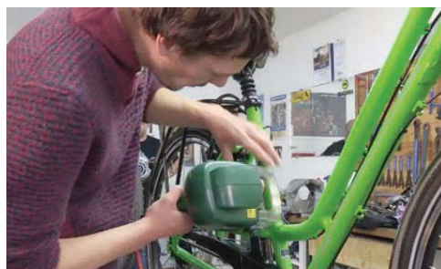
This French retailer is using a micro-percussion machine to engrave the registration number on a frame.
