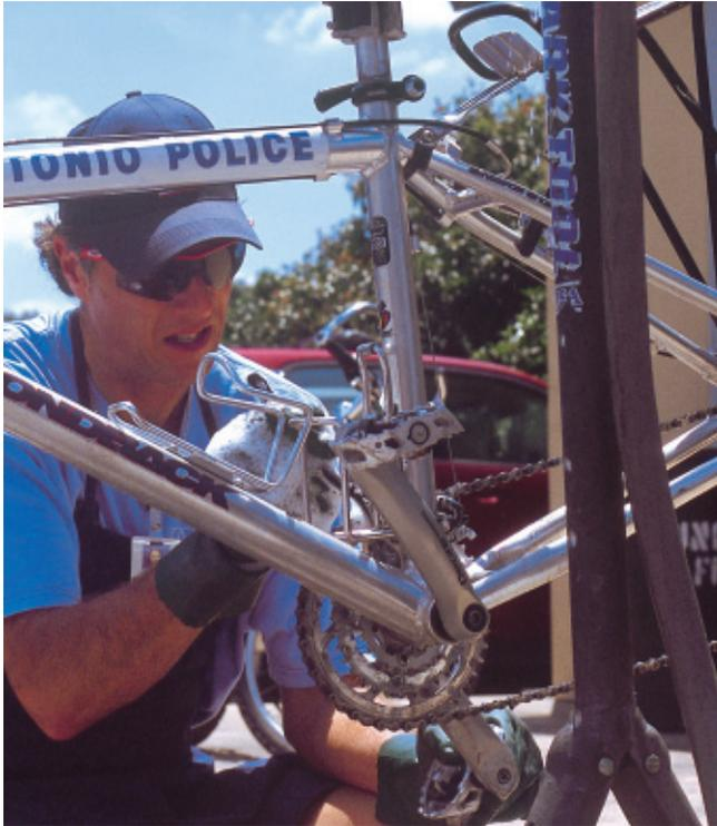
cannot be swapped from bicycle to bicycle. The brakes and drive train have fine-tune adjustments that are specific to each wheel, so it is important that they not be swapped. A malfunction of the brakes or drive train can result in serious injury to the cyclist, especially under critical use in an emergency response.
