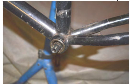
Accumulated sludge in the bottom bracket cartridge.
