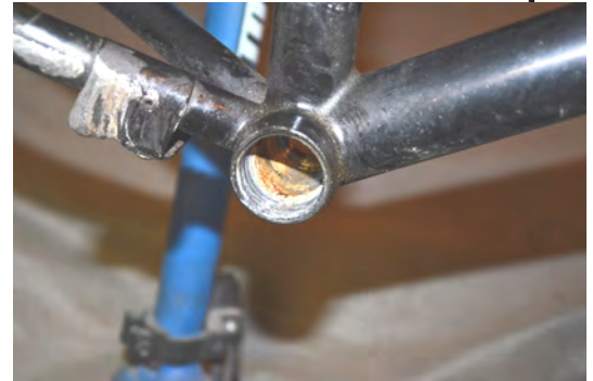
Inside the bottom bracket after removing the cartridge. Dried grease, dirt, some rust.
