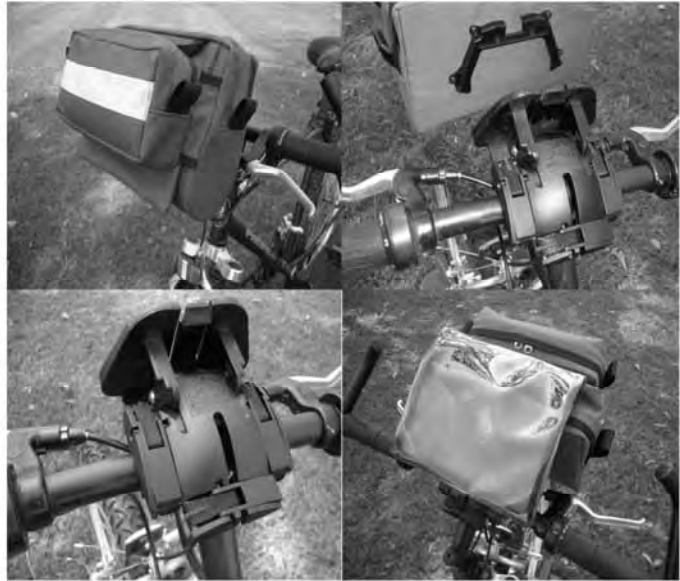
QUICK RELEASE LATCH ALLOWS FOR EASY REMOVAL
