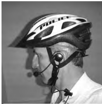
The Breeze headset, showing microphone position and headpiece position.
