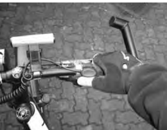
The handlebar mounted Press-to-Talk switch as fitted to my bike.
