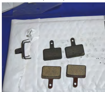
Worn disc brake pads (top); new disc brake pads (bottom).
