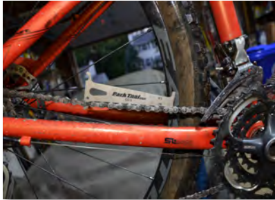
Checking chain elongation with a chain checker.
