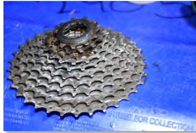
Rear cassette with uneven wear.
