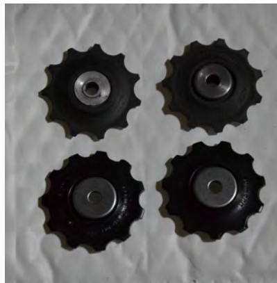
Jockey wheels: worn (top) and new (bottom).
