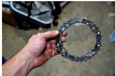
Middle chainring with excessive wear.
