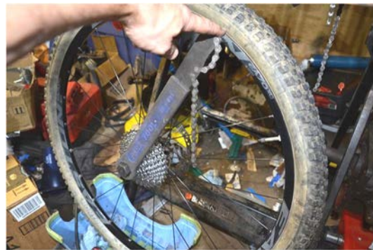
Tightening the lockring using the chain tool (9761)
