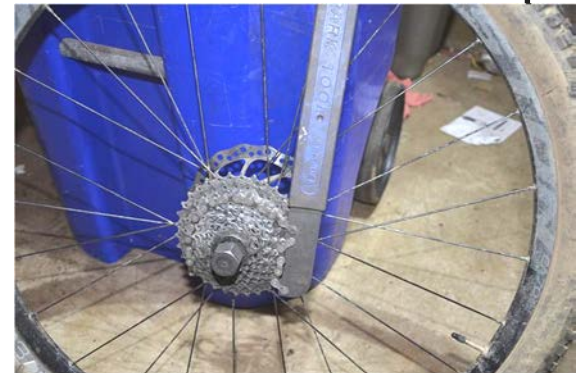
Placing the chain whip on the cassette (9721)
