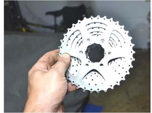
Back of cassette showing the matching splines (9759)
