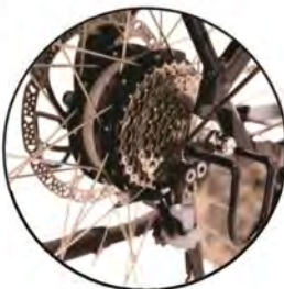
500 Watt Rear Hub Motor
