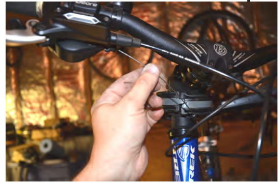
Rubbing the drop of oil along the length of the cable.
