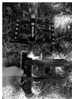
Standard pedal with toe clip vs the Catalyst
