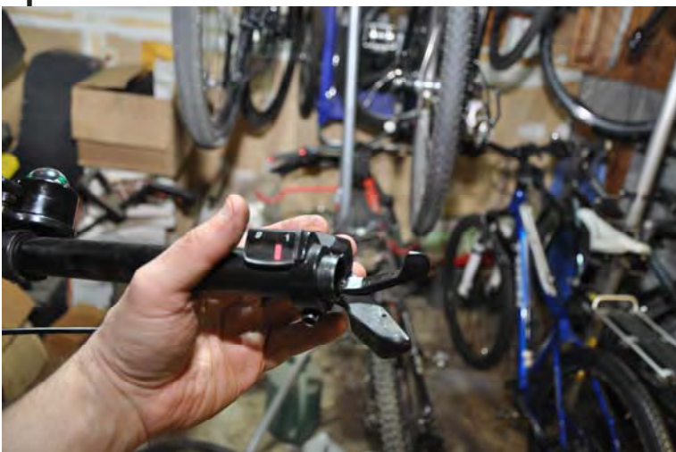
Installing the new shifter pod.
